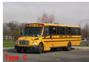
Type C Bus (Conventional) – These are based on a medium duty flat-back cowl truck chassis with the engine in front of the windshield and the entrance door behind the front wheels.
